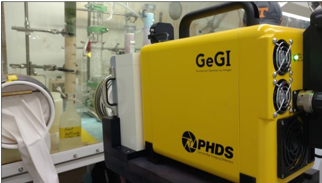
Figure 3.1: The GeGI v4 with Gray and White Lead Collimator and Black Tripod
